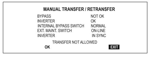
The message Retransfer to UPS or Transfer to Bypass will appear depending on status of the critical load. The operator has two choices: Either to accept OK or EXIT. If a transfer or retransfer is not allowed, the FLASHING message Transfer Not Allowed is displayed. Press EXIT to return to the MAIN MENU.
